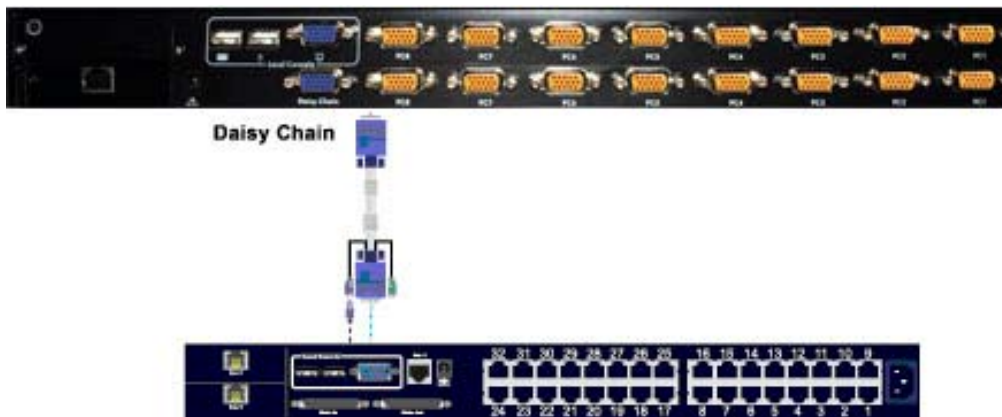
Figure 16. Daisy Chain through Computer Port
